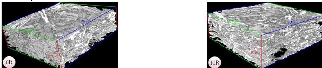
Figure 4: Microtomographs of handsheets produced from never dried (left) and ten times recycled (right) pulps. The sample size is ( $105 \mu\text{m} \times 350 \mu\text{m} \times 350 \mu\text{m}$ )
